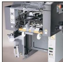
A chain delivery with automatically lowering, roll-away paper platforms is featured on the 9995s. A capacity of 17.3" (440 mm) lets the operator unload less often during long runs. When the delivery table limit is reached, a switch automatically shuts off paper feed so the stack does not overload.
