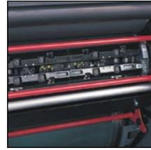
Our 9995C model features manual, straight-edge plate clamps. Positioning pins locate the printing plate into the proper position,
